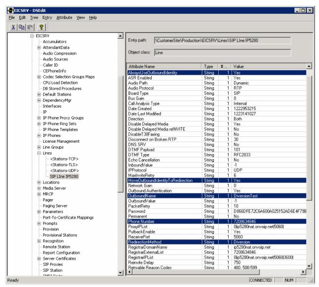
Figure 9: DSEditU Diversion Header For Forward/Follow Me Support
