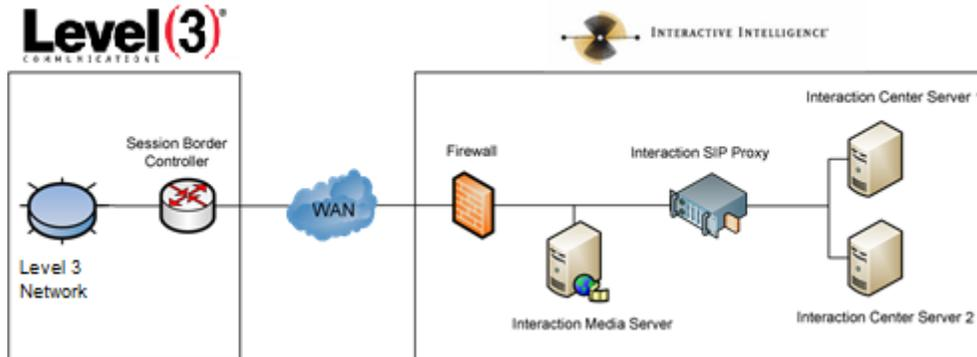
The external address of the firewall is the IP address given to Level 3 to verify the origination of the call, the customer, and services being supplied. As a reminder, Level 3 uses a static IP address to identify an end user and will deny the call if this IP address does not match.
